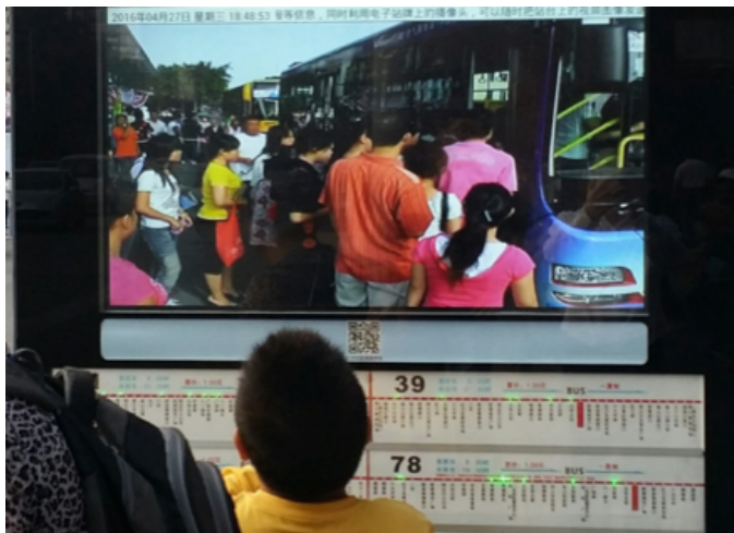
Fig. 1 A real-life snapshot of an electronic bus stop plate with information of real-time bus distribution along the bus corridor.
